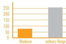
The overall vibration value determined from the frequency-dependent acceleration with a normal flange and the Rhoducer (measured with Bosch high-frequency angle grinder (2900 W) type number 0602331036, with grinding wheel 180 x 7,0 mm on GGG80 30 x 50 x 800 mm).
